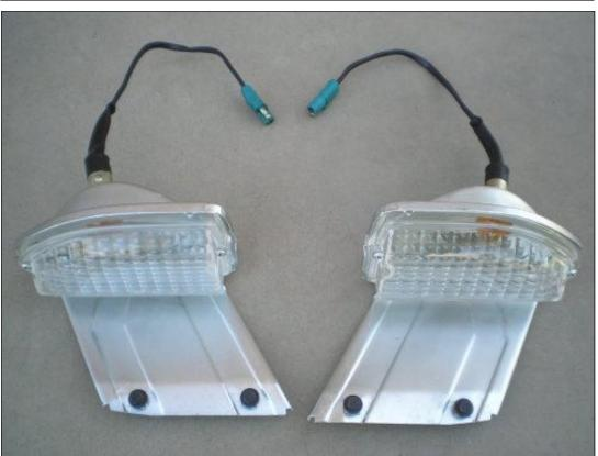
The inside of the housings were painted just like the 69 housings with reflective silver paint. Unlike 69 housings I have found no evidence of any date coding on the 70 housings as of today.
