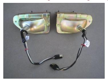
These housings were originally plated with a zinc dichromate from the factory with the wire harness socket having the same finish. These housings are actually two stamped pieces that typically had 5 spot welds holding them together.
