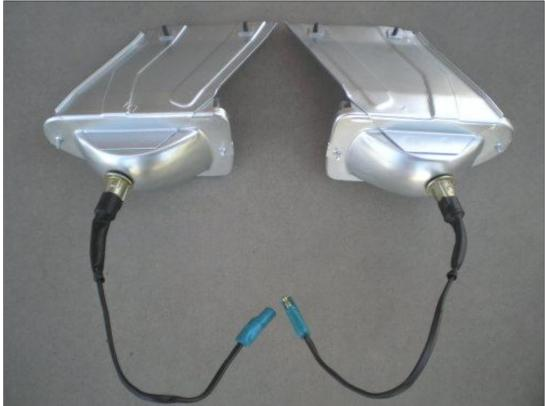
These housings were originally plated with a silver zinc from the factory with the wire harness socket having a zinc dichromate finish. As with 69 housings, these are actually two pieces that typically had 5 spot welds holding them together.
