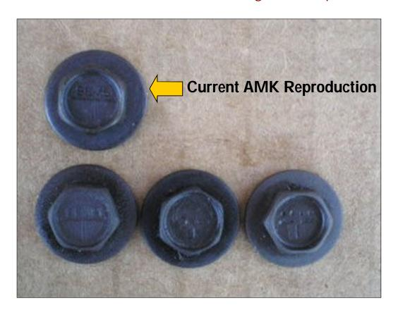
1969 and 1970 ΑII housings are attached to the bumpers with two 8 -32 x 3/4 screws that would have had a phosphate finish ing. Ford part number 57077-S. There are different style three head markings on original housings I have come across and AMK makes a copy of the most popular head marking with the SEMS stamping.
