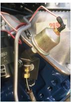
39 The oil sender set up is different for cars with and without a tachometer. For cars with a tach the oil sender is threaded directly in to the engine block as shown on the top left. For a non-tach car because the oil sender is so large a special bracket and tube was used to mount the sending unit next to the coil.
