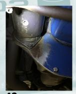
**42** The cover on the rear of the motor is painted blue except where the starter mounts. This area was left bare to ensure a good ground.
