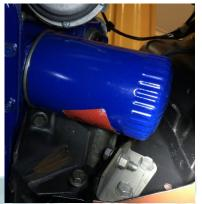
**40** Original Autolite FL-1 oil filters used in 1969 and 1970 would typically have a single crimp on the top of the oil filter, although some early 1969 cars could have a dual crimp style. All of them have date codes and this one here on the left decodes as February 4, 1970. Original factory oil filters where blue and also had date codes stamped on them.
