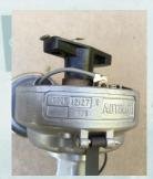
**20** The Boss 302 has a dual point distributor with a C9ZF 12127 cast in the back of the housing. This would be dated as well as in this example here the 9J8 is Sept 8 1969. Typically a paper tag was placed over front as shown here.
