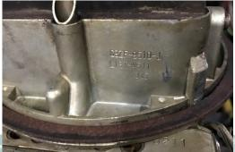
**12** The carburetor used on a Boss 302 is a 780 CFM Holly. In 1969 it was a C9ZF-9510-J and in 1970 was a D0ZF-9510-Z. The date code shown here above is 935 which decodes as 1969, 3rd month, 5th week.
