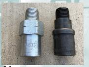
**41** The PCV valve used in 1969 and until February 5 1970 was marked with the engineering number C70Z-6A66-A (EV-42), and shown above on the left. After that a D0OZ-6A666-A marked unit (EV-51) was used shown on the right.
