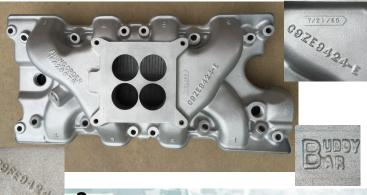
3 The original assembly line intake manifolds are aluminum with some slight blue overspray on the front and backside from when the motor was painted. Two engineering number versions exist which are a C9ZE9424-E or a C9FE9424-E. The underside of the intake has a casting that says BUDDY BAR. Date codes (when present) are on the front next to the engineering number.
