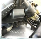
**13** The original accelerator pumps had a square body as shown above and the later replacements had the round style thinner body. This is visible on the front of the carb when mounted on the intake manifold.
