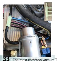
that was used on the Boss 302 motor is shown here and is a "5 way" T. However, this was not the only version used as some may have a 4 way or a combination of 2 way vacuum T's used.
