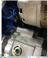
46 The engine OK stamp is typically seen in 1969 on the cast iron smog pump bracket, and in 1970 on the actual cylinder head as shown here. This is different than the OK valve cover stamp.
