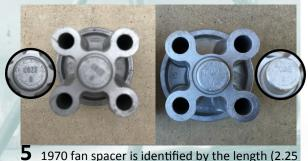
inches) and engineering number stamped on the nose (DOAE-A). The 1969 spacer is different and
