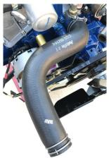
The upper radiator hose is ink stamped with the engineering number C9ZE-8B274-C and the lower is ink stamped with DOZE-8B273-B. Note the band style clamps are stapled in place and the "alligator" texture on original hoses.
