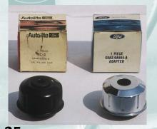
35 The 1969 Boss 302 used the chrome C8AZ-6766-B breather cap. In 1970 the cap was used on Dearborn built cars while Metuchen also used the black breather cap C8AZ-6766-A.
