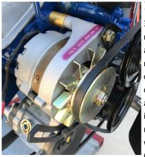
**1** The 1970 Boss 302 alternator is rated at 55 amps, as indicated by the red dye on the top of the housing. The dye was actually applied to the housing before the engineering numbers were stamped on (DOZF-10300-A) so
