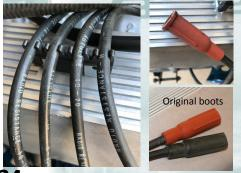
**34** Spark plug wires were Autolite with either orange or black boots as shown. Note the original boots shown here with no ring on the ends as compared to the style seen with the ring used on other applications. The wires are date coded 1Q-70 which is first quarter of 1970.
