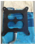
**26** The carb spacer is installed with the elbow towards the front of the motor. This early NOS piece is brown and later service pieces were black.
