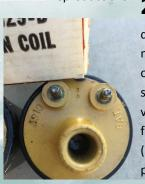
**28** The ignition coil used on the Boss 302 motors was an Autolite yellow top coil. Original coils typically have a mold number cast between the two terminals on the top of the coil as shown.
