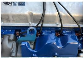
31 Notice the engine hook is a slightly lighter shade of blue than the motor. That is because they were painted at an outside shop. There is a slight amount of blue overspray from the motor on the very top edge of the engine lift hook. There is a special thin nut used to hold on the engine lift hooks as shown in phosphate finish.
