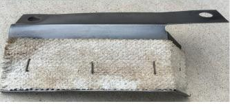
11 The engine mount heat shield was never serviced by Ford and is only used on the drivers side of the Boss 302 motors. It is a bare piece of stamped steel with an asbestos strip that is stapled to it in place. Shown above uninstalled and installed for reference.
