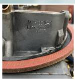
**51** The original air cleaner to carb gasket, was a C5ZZ-9654-B and was .18" thick. It was covered on one side with a red dry glue and was intended to be installed as shown facing up. This was done to prevent it from falling off during removal. Once the motor was heated up this gasket would stick to the bottom of the air cleaner.
