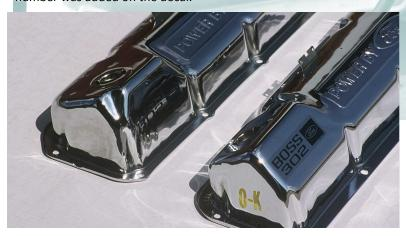
**6** All 1969 Boss 302's had the chrome valve covers installed that are stamped with Power by Ford. Some early 1970 Boss 302's also had chrome valve covers installed which are slightly different. The two versions are shown here with the 1970 version shown on the left. All other 1970 Boss 302's received the finned aluminum valve covers which were also the only replacements ever sold by Ford.
