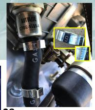
38 The flexible rubber fuel lines shown above with the correct original style fuel line clamps—spring clamps with square tabs at the fuel pump, and crimp style at the carb marked with .590 and an "E" for the manufacturer. Earlier fuel lines were marked with a C.
