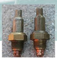
17 The ported vaccum switch that is mounted in the thermostat housing was a C8AE-A version for 1969 and a D0AE-A for 1970. The change over date was approximately Aug/Sept 1969. Date codes are a month year format with the middle character representing the manufacturing plant—H for Hanover IL and K for Kalamazoo MI.
