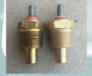
15 The temperature sender used on a 1970 Boss 302 would have a red insulator as shown and be stamped Autolite 260 with the date code. A 1969 Boss 302 has a green insulator and is stamped Autolite 258 with the date code. The format for the date would be month/year. Later versions were stamped Motorcraft.
