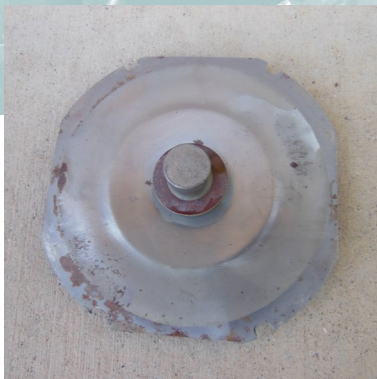
The steel diaphragm
