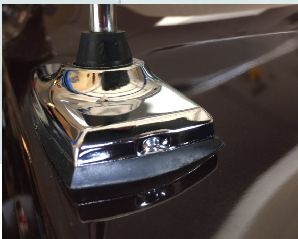
Mustang antenna and gasket installed
