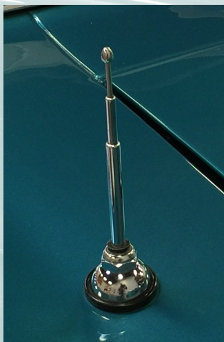
Original Shelby antennas could have a spear shaped or round ball on the tip of the antenna mast as shown here.
