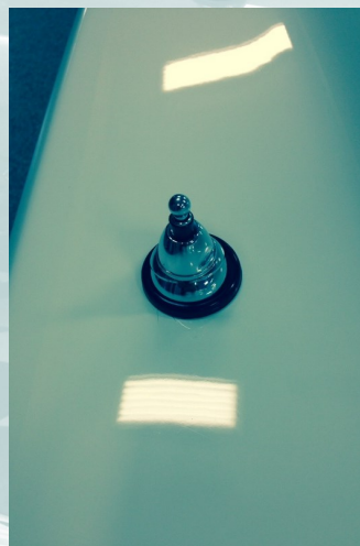
Original Shelby antennas could have a spear shaped or round ball on the tip of the antenna mast as shown here.
