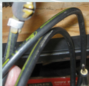
Ink stamp markings on the original 200 inch antenna lead wire.
