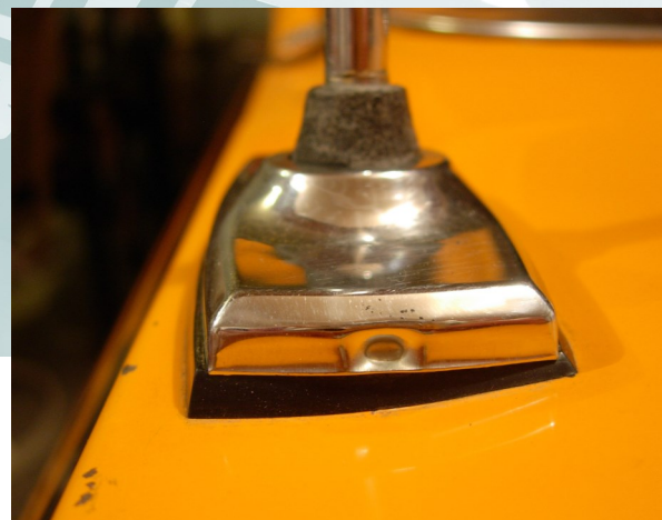
Cougar antenna and gasket installed
