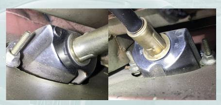
Installation of left and right side of the reverse lights on an unrestored low mileage 1968 Mustang. Shown here is what is typical for the hardware and note the distinct L and R for the right and left side assemblies that can be seen
