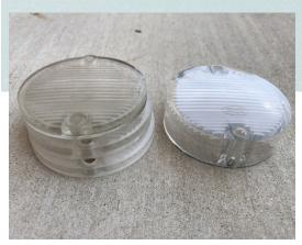
**Left:** Shows the single stacked lenses as compared to the thick lens that was used from April 69.
