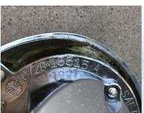
The 1969 and the 1970 model year Ford used exactly the same housing as the 1967/1968 versions, as they are still marked with C7ZB engineering numbers. There was really only two major changes. First was the wiring harness assembly which now has a red connector on the end and the wires are covered in a black polyvinyl chloride insulator and marked with a C9ZB-15536-B. The second change is in the design of the reverse lamp lenses which are now marked with a SAE-R 69MG.
