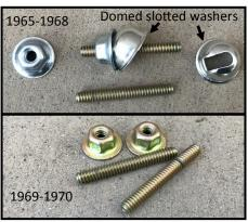
1965 to 1968 applications normally use the domed slotted washer, and 1969 to 1970 does not, even though this washer is still shown in the assembly manual. Unrestored cars (69-70) never seem to have these washers installed.
