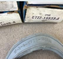
**1967—1970** The second version of back up lamp gaskets were used on all 1967 to 1970 model year Mustangs. Note the correct grey color as assembly line originals had since there is some Ford service replacements that were done in black. The gaskets are now the same for the left and right side and marked with a C7ZB-15533-A, also with a cut out for the drain.
