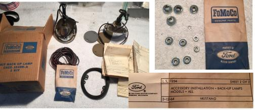
For owners that wanted to add reverse lights on their 1964 1/2 and 1965 Mustangs Ford sold a *Back Up Lamp Kit* under the service part number of C5ZZ-15499-A. This kit included everything from the template to cut the rear valance, to all the wiring, the reverse lamp assemblies, gaskets, screws, lenses etc. Then in 1966 this became standard equipment.
