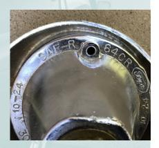
The right hand assemblies are marked in the cast housing C4ZB-15515-B and the left hand assemblies are marked C4ZB-15A509-B. The wire harness is ink stamped with C4ZB-15536-A and FoMoCo and is two wires molded together with a spade and bullet end connector with the light bulb socket finished in a zinc dichromate. Note the smaller drain hole on the bottom of the housing as compared to the 1967 to 1970 versions.
