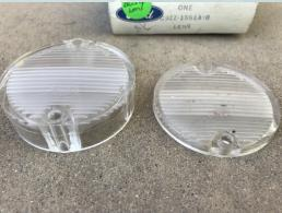
Three different lenses were used from 1965 to 1970. The first lens was used until the end of model year 1968 and is marked with SAE R 64 CR. The second and third lenses are marked the same with SAE R 69 MG with the only difference being the thickenss of the lens as described on the previous page.
