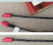
A super rare find, Ford actually serviced just the entire wire harness and socket assembly. Shown here the C9 versions with the red plugs.
