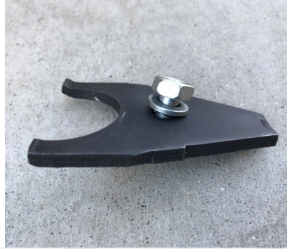
17 An original style distributor hold down (B8A-12270-A) is shown here with the correct installed position (tang's up) and a phosphate and oil finish held in place by a zinc hold down bolt and lock washer.
