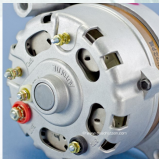
Rear housing detail showing the AUTOLITE stamping and the commonly referred "tear drop" center.
