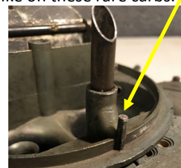
Original style square accelerator pump. Visible from front when installed and mounted on intake.
