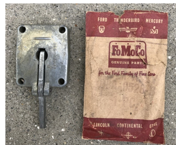
Original style square accelerator pump. Visible from front when installed and mounted on intake.
