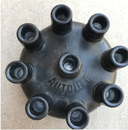
16 The correct original distributor cap has AUTOLITE cast into the top of the cap as shown here and is a black molded piece.
