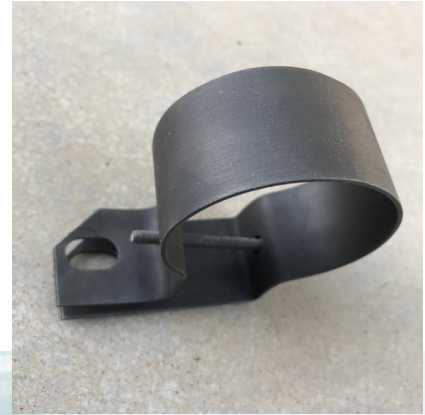
18 The correct style ignition coil bracket assembly. Note the position of the notch that fits against the intake manifold and the correct finish.
