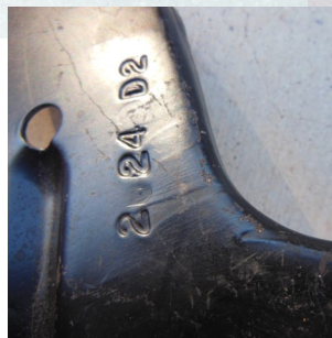
Paint runs visible
