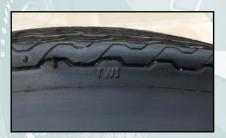
**Safety Warning.** None of the original tires had the Safety warning that is required on all new tires today. This started to be used in about 1980 so was never seen on the original 1960's and 1970's tires. Usually stamped on the back side of the tire—examples shown here.
