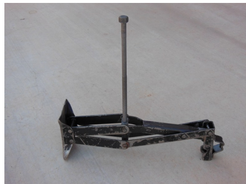
Pictured here on the left is the method in which a jack would be dipped in paint before being assembled. The threaded portion of the drive screw at times would have been coated with grease to protect from paint. Afterwards it would be assembled.
