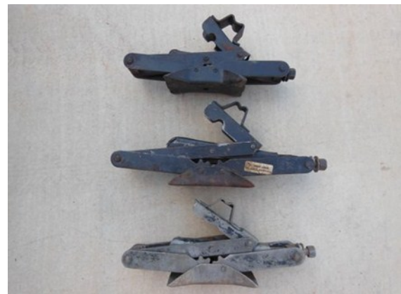
Side by side comparison with the first generation (top), second generation (middle) and Maverick jack (bottom).
