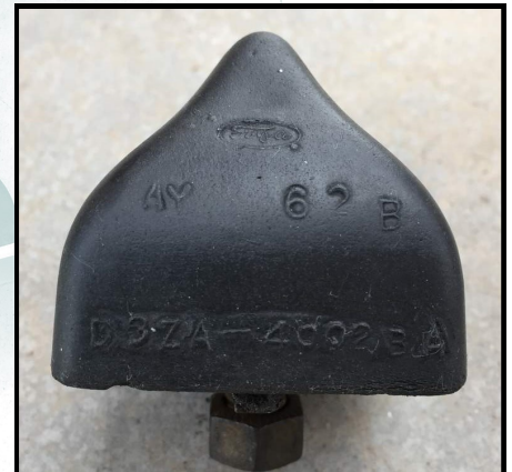
D3 with coarse thread stud, used from 1973 on and as service replacements.
