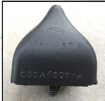
C9 with coarse thread stud, used from 1969 to 1973.**
