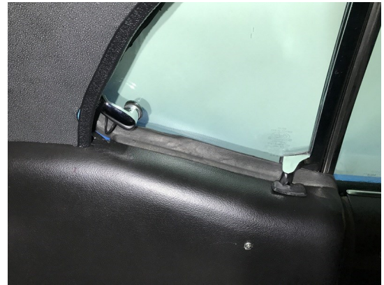
1970 The change in the cut out area no longer requires the quarter window cap anymore. This 1 inch difference eliminates the need for this added piece.
