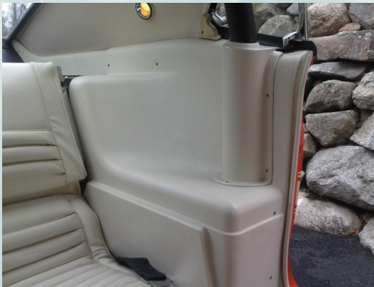
1969 Shown here with the quarter window cap to cover the cut area of the panel. This piece is not used on a 1970.
