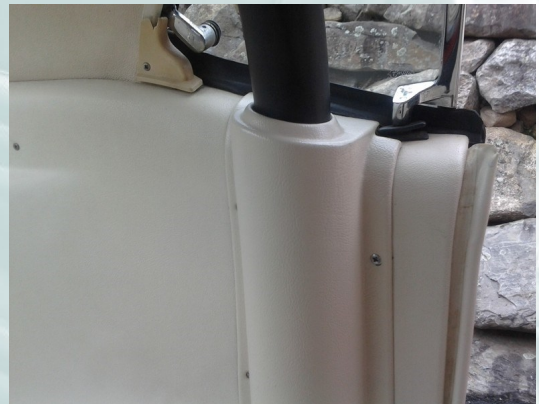
1970 The change in the cut out area no longer requires the quarter window cap anymore. This 1 inch difference eliminates the need for this added piece.
