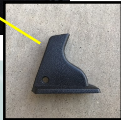
1969 Shown here with the quarter window cap to cover the cut area of the panel. This piece is not used on a 1970.
