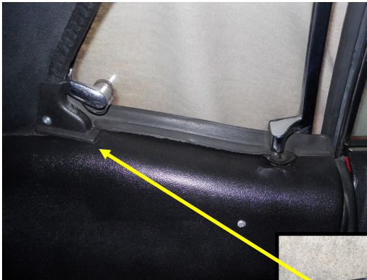
1969 Shown here with the quarter window cap to cover the cut area of the panel. This piece is not used on a 1970.
