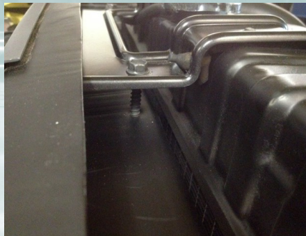
Lag screw shown installed shown from the side on a Dearborn Boss 302.
