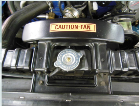
Upper radiator bracket on Boss 429 with additional finger guard installed.
