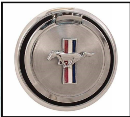
DOZZ-9030-D pop off style cap that was used with the 1970 Mach 1 package also had the longer neck to accommodate the CA emissions package.
