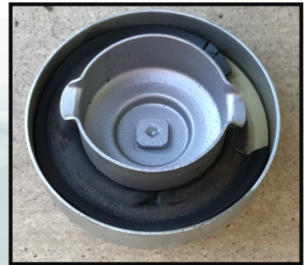
Inside of the DOAZ-9030-A cap showing the longer neck.
