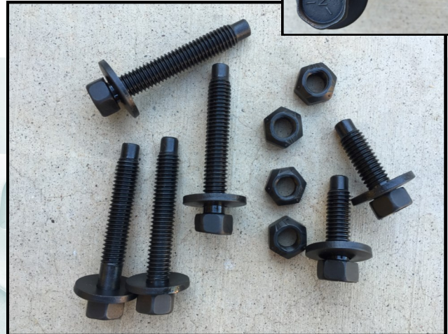
Bolts with captive washers typically seen on Dearborn and Metuchen cars.
