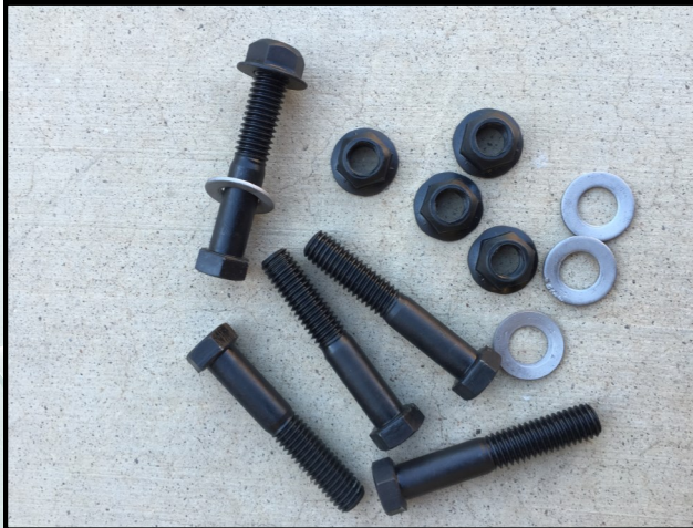
Bolts with separate washers typically seen on San Jose cars.
