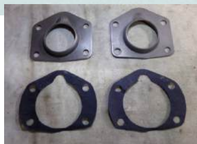
COAW-4020-B bearing retainers with matching gaskets 1965-1968
