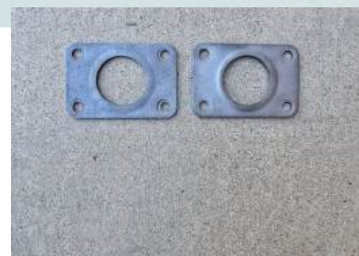
C8UZ-4020-A bearing retainers. These are used with no gasket. 1968 –1973
