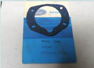
Gasket used between bearing retainer and backing plate A8AZ-1001-A used till 1968
