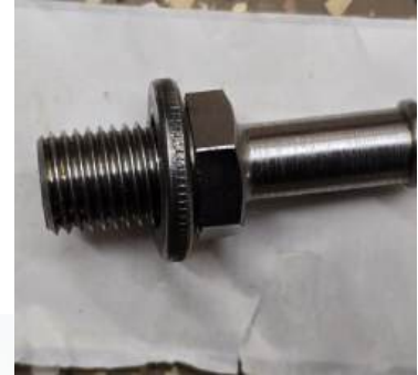
Split lock washer used 1967 to 1973. Not unique serrated edge
