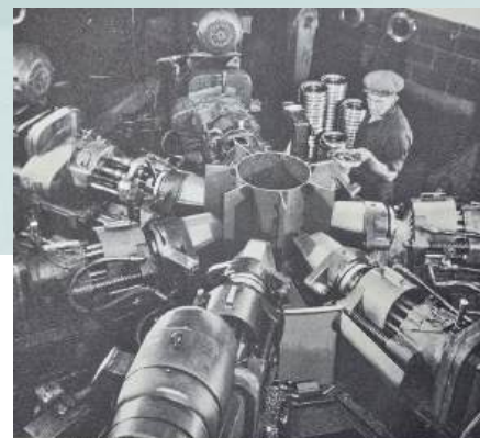
Multi-station drilling and tapping machine which drills, chamfers and taps holes in back of ring gears.
