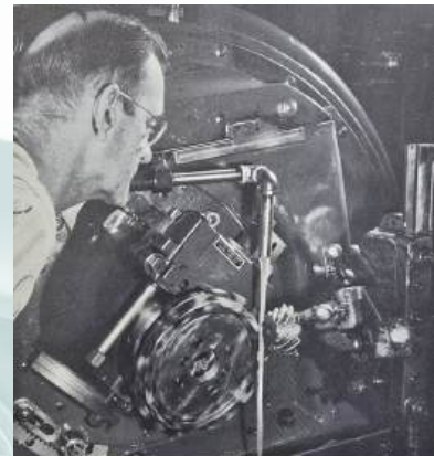
Checking a pinion finisher
