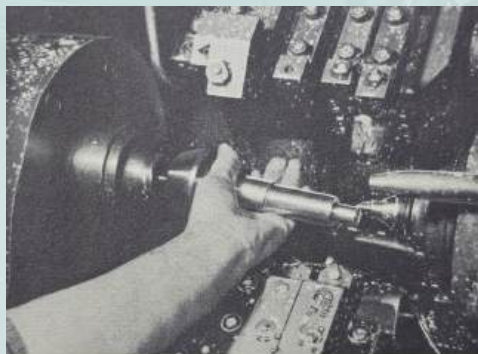
Drive pinion blank being removed from the high speed turning lathe. Thirteen carbide tools turn forging to accurate dimensions at a cutting speed of nearly 1,300 surface feet per second removing three pounds of metal in 15 seconds.
