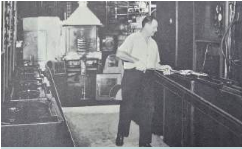
Hot ring gears are removed from furnaces and oil quenched in a press to prevent distortion.
