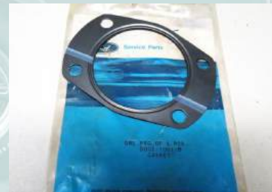
Metal gasket used between backing plate and axle housing D00Z-1001-A used from 1970 to 1973
