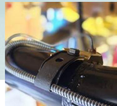
Typical installation showing the bracket in place holding the brake line.
