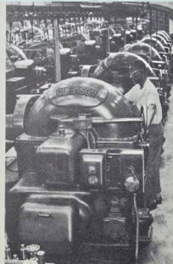
64 machines finish cut the teeth in the drive pinion to the size and shape required (32 machines generate the drive side of the teeth and 32 generate the reverse side).
